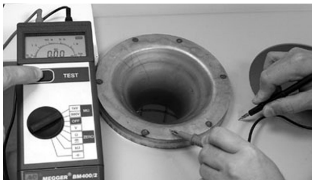
Top load collector: testing resistance between cage and tubesheet.
